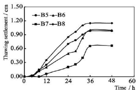
Figure 14: Conventional canals thawing settlement in a closed system 10.
