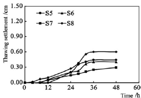
Figure 13: Soilbags-treated canals thawing settlement in a closed system 10.
