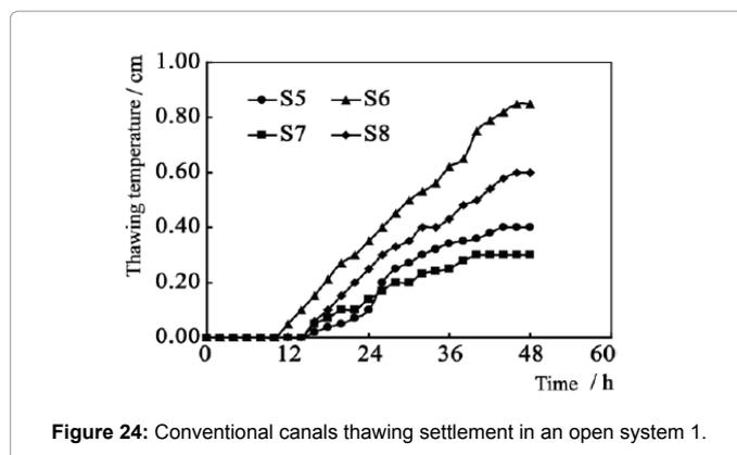
Figure 24: Conventional canals thawing settlement in an open system 1.
