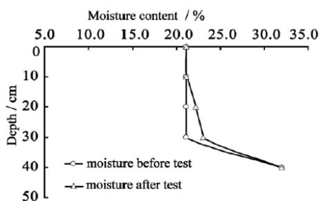
Figure 19: Soil bags-treated canals moisture content in an open system.
