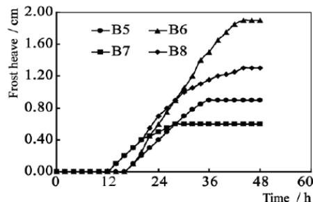
Figure 16: Conventional canals frost heave in an open system 1.
