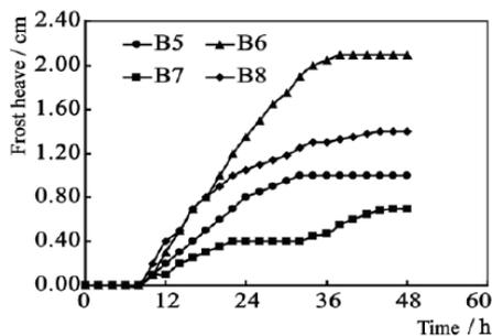
Figure 18: Conventional canals frost heave in an open system 10.
