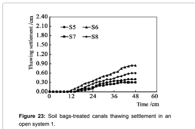
Figure 23: Soil bags-treated canals thawing settlement in an open system 1.
