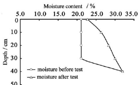
Figure 20: Conventional canals moisture content in an open system.
