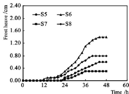
Figure 17: Soil bags-treated canals frost heave in an open system 10.
