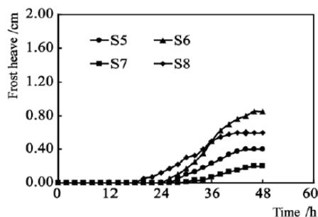
Figure 15: Soil bags-treated canals frost heave in an open system 1.
