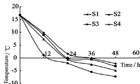
Figure 21: Soil bags-treated canals temperature in an open system.
